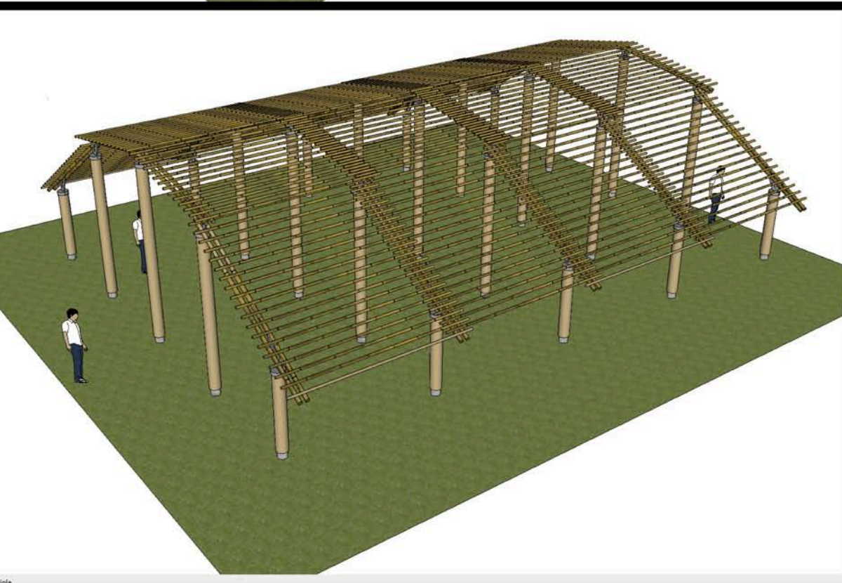
A series of carbon composite tubes are used as columns to support a bamboo ceiling frame structure over which solar membrane is draped over to provide shelter from the rain and satisfy all electrical and power needs.
