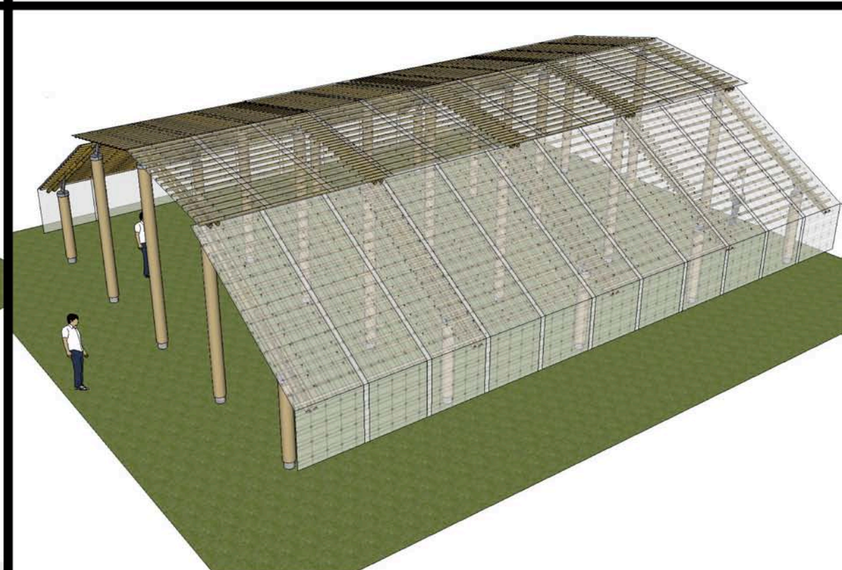
A series of carbon composite tubes are used as columns to support a bamboo ceiling frame structure over which solar membrane is draped over to provide shelter from the rain and satisfy all electrical and power needs.
